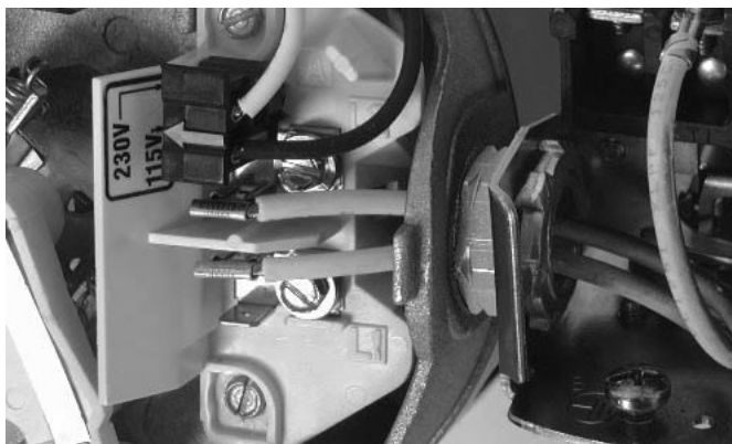
Figure 7 - Voltage set to 115 V, Plug Type
