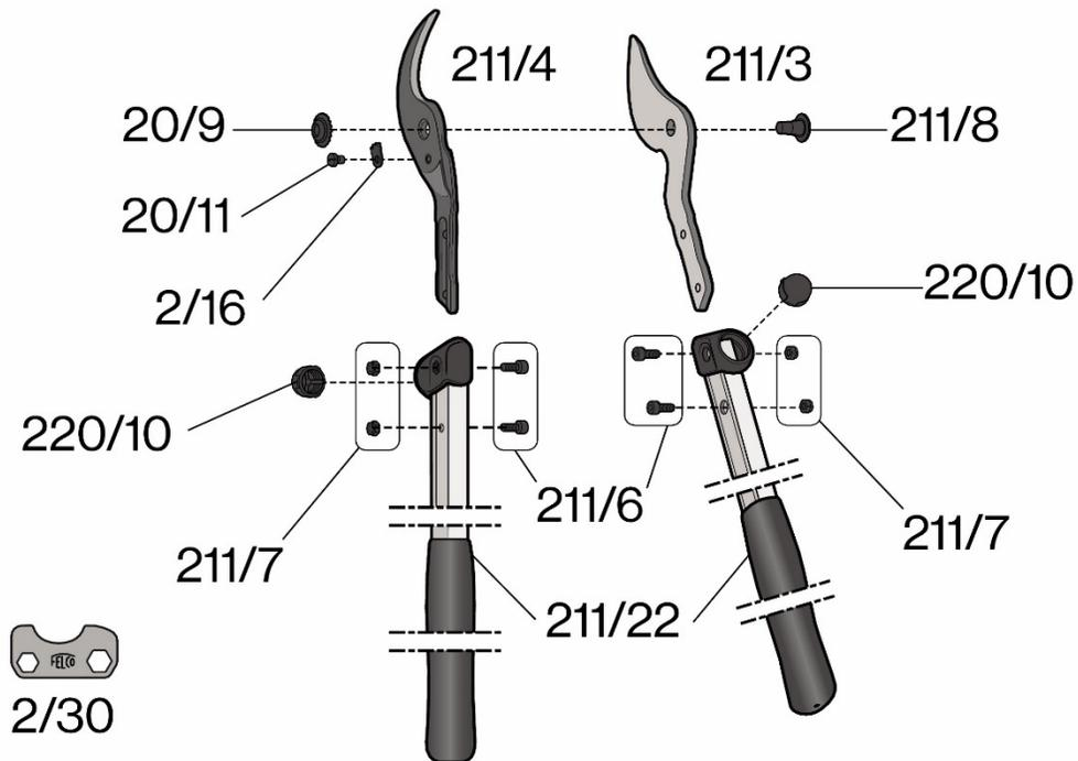
\*New lopper line parts are interchangeable except for the handles parts 211/22, 211/32, 211/42
