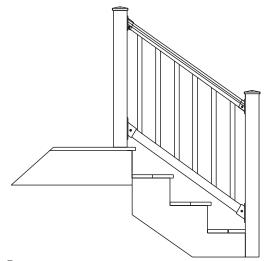
With rail mounted in place, measure and mark post sleeves. Cut post to height with a saw and clean edge of cut. Apply a small bead of silicone to the inside edge of post cap and install on top of sleeve (let set 12 hours for adhesive to cure).
