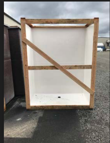
Diagonal board is used on 5 foot shower stalls for added protection
