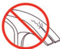
Crack in claw section
