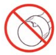
Chips or dents on face
