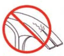
Crack in claw section
