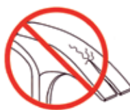
Crack in claw section
