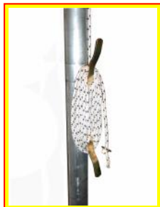
Rope Lanyard Elevating Mechanism
