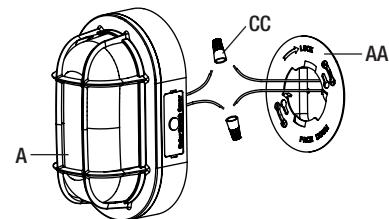
**4** Align the side slots on the fixture body (A) with the mounting bracket (AA) and fix the fixture body (A) securely by carefully rotating in clockwise the side slots inside the mounting bracket (AA).
