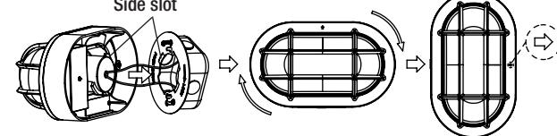
**5** Apply silicone sealant (not included) between the fixture body (B) and the wall for additional protection against water and dust. Restore power at the electrical panel. Turn on the light switch to activate the fixture.
