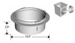
**Uses:** Use to attach 8" & 10" singlewall pipe to 9", 12" square DrainTech basin and low-profile drains where an offset connection is needed. Reduces 8" pipe to a 6" opening.
