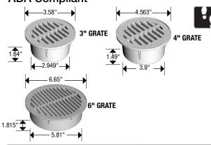
With: 3", 4" & 6" corrugated single wall and dual wall pipe, SDR 35, 2729 S&D and TripleWall pipe. All 6" grates may be used with 6" round basins.
