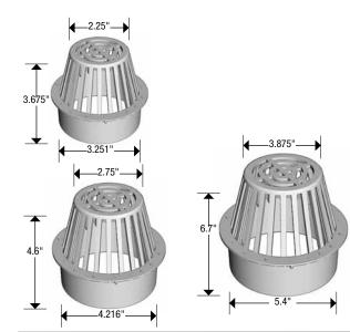
**Use With:** 3", 4" & 6" corrugated single wall and dual pipe, SDR 35, 2729 S&D and TripleWall pipe. All 6" grates may be used with 6" round basins.
