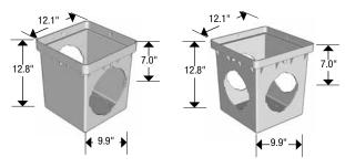
**Use with:** 3", 4", 6", 8" corrugated singlewall pipe; 3", 4" TripleWall pipe; 3", 4", 6", 8" SDR 35 pipe; singlewall HDPE fittings; DrainTech 12" square riser; DrainTech Universal End Plug and DrainTech offset adapters.
