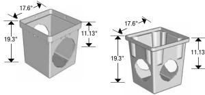
**Use with:** 3", 4", 6", 8", 10" corrugated singlewall pipe; 3", 4" TripleWall pipe; 3", 4", 6", 8", 10" SDR 35 pipe; singlewall HDPE fittings; DrainTech 18" square riser; DrainTech Universal End Plug; 2 reducing rings included.
