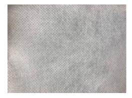
DeWitt Supreme (or N-Sulate) is a 1.5oz spunbond polypropylene fabric used primarily for plant protection. N-Sulate is formulated to resist uv degradation, and allows air and water to pass through the fabric.
