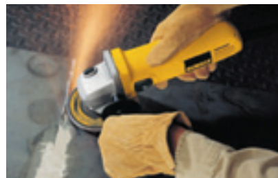
Metal fabricators use flap disks for all types of metal finishing, deburring, edge blending, chamfering and surface preparation.
