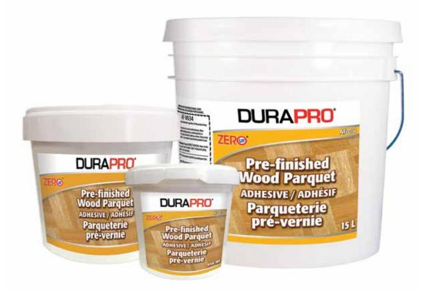
DURA PRO AF 0034 is a high solids latex based adhesive used for direct glue-down of pre-finished 12"x12" finger strips mosaic parquet made of maple, oak or birch on T&G floor grade plywood or cured concrete either on above or below grade.
