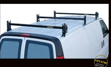
High-strength I-5/8" diameter telescoping steel racks adjust to fit different width fullsize vans with rain gutters. Heavy-duty mounting brackets allow positioning the cross bars at different heights to provide proper clearance and reduce wind noise. EZ-mount Clamps secure the brackets on the rain gutters. They are easy to install or remove. Use 3-Bar Rack for more support of longer or heavier loads.
