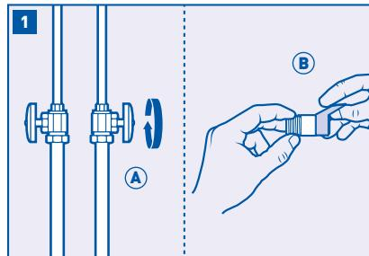
Turn off water supply (A) and open nearest faucet to drain pipes before installation. Apply about 6" of Teflon® tape (B) in clockwise direction to pipe threads of each adapter.
