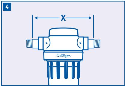
Measure overall length of configured system with adapters attached.
