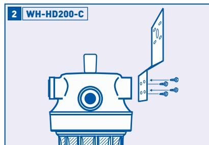
If using optional BR-C mounting bracket, start by making sure the arrows facing you on the system are consistent with the direction of your water flow. If necessary, remove filter life indicator holder if on the back side of the unit, and move it to the front. Align the holes of the bracket with the holes on the back of the filter head. Insert four mounting screws through the bracket and into the filter head until tight. Otherwise skip to step 3.
