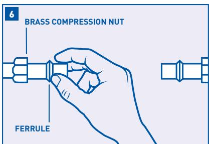
Slip brass compression nut and ferrule onto each end of 1" pipe.
