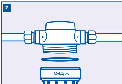
Lubricate O-Ring with a coating of clean food-grade silicone grease. Insert O-Ring back into groove and smooth into place with finger.
