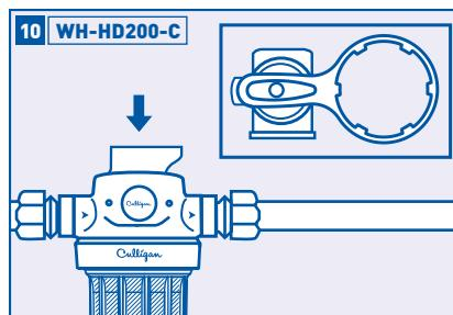
Ensure the filter housing has been properly tightened using the housing wrench provided. Turn bypass valve to "Filter" mode using wrench, then slowly turn on main water supply. Slowly press red pressure-relief button on top of filter to release trapped air. Check for leaks. Open nearest faucet and flush filter cartridge for 5 minutes. Reset filter life indicator (hold reset button for 2 seconds).
