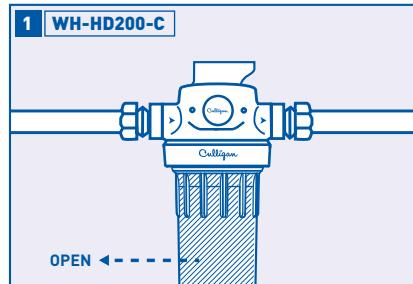
Turn water off by rotating bypass valve to "Off" or "Bypass."
