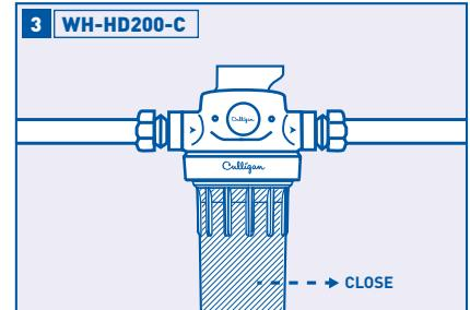
Screw the bottom of housing onto the cap until tight. **DO NOT OVER-TIGHTEN.** Make certain standpipe in filter head slips into cartridge.
