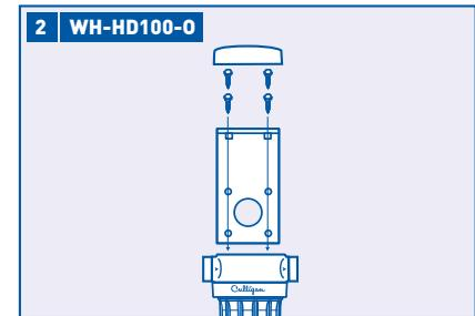
If using optional BR-0 mounting bracket (sold separately), start by making sure the arrows facing you on the system are consistent with the direction of your water flow. Remove head cap and align the holes in the bracket with the holes in the filter head. Insert four mounting screws through the bracket and into the filter head until tight. Replace head cap. Otherwise skip to step 3.
