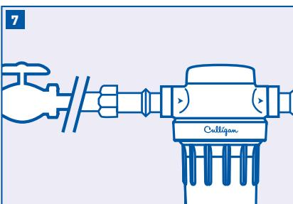
Align filter assembly with ends of pipe, making certain your water flow is in the same direction as the arrows on your filter head. It will be necessary to spread ends of pipe apart to install filter assembly. Using two adjustable wrenches, hold incoming fitting securely with one wrench and tighten nut with second wrench. Repeat process for outgoing fitting.
