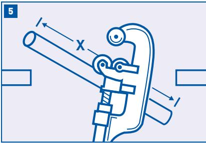
Using a pipe cutter or hacksaw, cut and remove marked section of pipe. File or sand sharp edges on remaining pipe.
