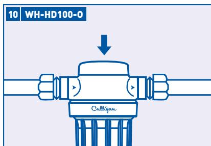
Ensure the filter housing has been properly tightened using the housing wrench provided. Slowly turn on main water supply. Slowly press red pressure-relief button on top of filter to release trapped air. Check for leaks. Open nearest faucet and flush filter cartridge for 5 minutes.
