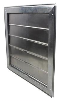
Cool Attic® Power Gable Vents require a MINIMUM 600 sq inches NFA of intake ventilation. Inadequate intake ventilation will lead to motor failure.
