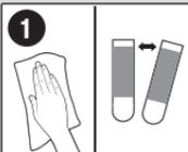
**1** CLEAN surface with isopropyl rubbing alcohol, wipe gently, let dry. Do not use household cleaners. SEPARATE strips.
