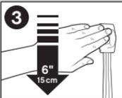
**3** STRETCH STRAIGHT DOWN ALONG WALL AT LEAST 6 INCHES (15 cm) until strip releases from wall.
