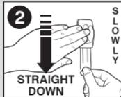
**2** Hold clip gently to prevent clip from snapping fingers. DO NOT press clip against wall.
