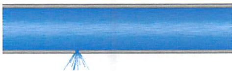
Refrigerant and oil are drawn to the leak site where they eventually escape into the atmosphere.
