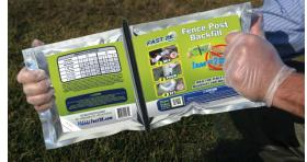
Fast 2K is a two-part proprietary polymer that expands to fill the peripheral void between a fence post and the hole. Fast 2K expands immediately after mixing and holds the posts in 2-5 minutes. Fences can be built in 15-30 minutes after Fast 2K finishes expanding.
