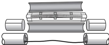
**1.** Carefully cut out damaged section up to 10 feet. Larger sections can be accommodated using multiple repair kits.
