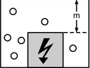
$\Delta \Delta \dots m$ Protected against effects of prolonged immersion under pressure |
