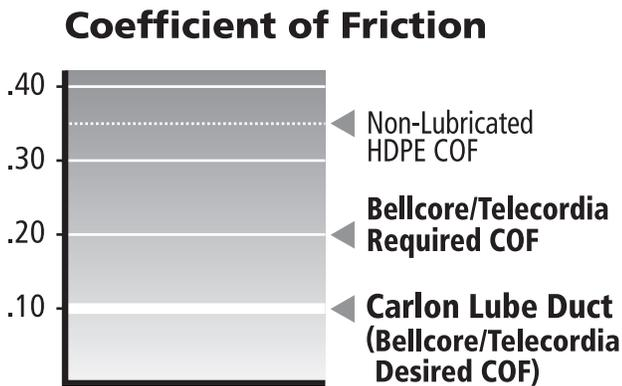
Coefficient rating based on Bellcore/Telecordia GR-356-CORE for optical cable innerducts.
