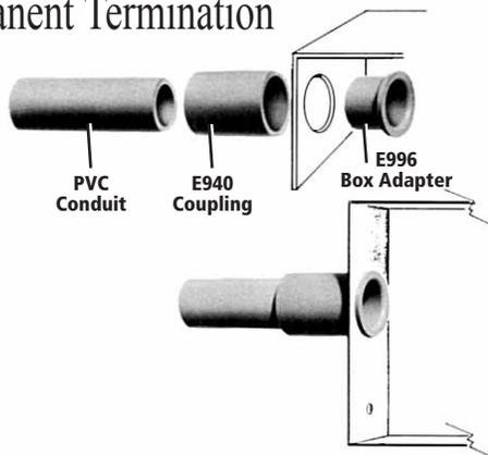
Apply solvent cement to shoulder and shank of box adapter and insert through knock-out from inside the enclosure. Push coupling over the shank of the box adapter, tight against the enclosure wall. Rotate the coupling about one-half turn while installing, and hold in position for a few seconds to permit setting of solvent cement. The coupling is now ready for the conduit to be installed. Only the shoulder of the box adapter extends inside the enclosure.
