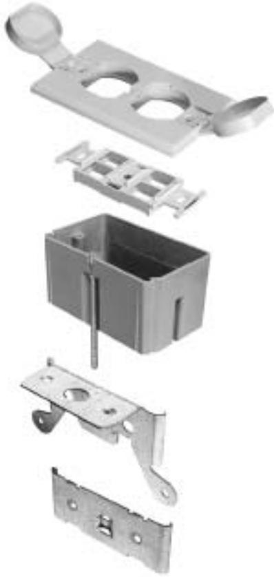
The Carlon Low Voltage Adjustable Floor Bracket is specifically designed for the low voltage, structured cabling market. . . *the floor bracket is industry standard orange to identify low voltage applications, the open design provides the space needed for low voltage bend radius requirements, and the Leviton QuickPort® Quad 106® Insert provides up to four low voltage outlet ports.* The Carlon Low Voltage Adjustable Floor Bracket is ideal for any residential or commercial low voltage application.
