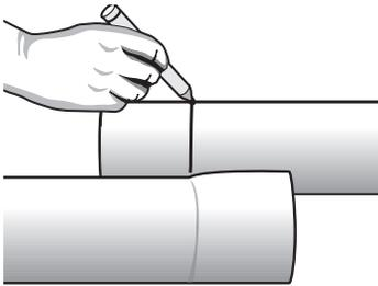
**1.** Lay the Multi-Gard sections side by side and mark the male end at the base of the bell on the female end. Make a straight cut using a standard carpenter saw.
