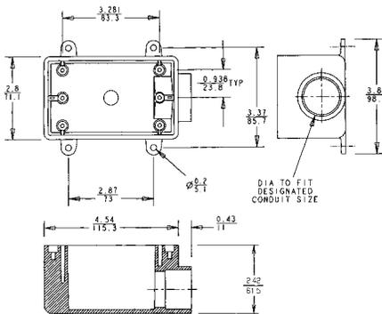
For dead-end terminations where large devices or additional wiring capacity is required.
