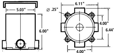
Carlson Round Floor Boxes allow for various thickness of concrete pours. Trim out is easy – just use a handsaw to cut off box at desired height to accommodate carpet, tile, or other flooring. Carlson leveling ring guarantees a level top every time, even if the box is tipped slightly during the pouring process.
