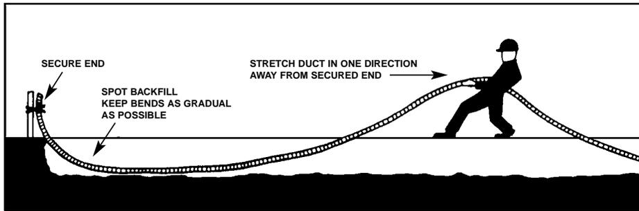
top of the conduit is recommended. After final backfill is placed, tamping may be used to finish the grade.
