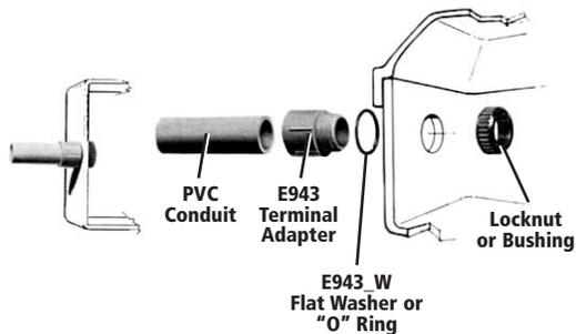
If watertight construction is required, place flat washer over the threads of the terminal adapter, securely against the shoulder. Insert the adapter threads through knock-out and secure using either a standard locknut or threaded bushing. If watertight construction is not required, eliminate flat washer.
