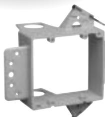
Open-backed to easily accommodate the bend radiuses required for low voltage cabling and deep devices such as volume controls, and is designed to fit a standard two-gang faceplate. It also features an easy nail-on mounting or screw-in bracket, while more hard shell provides increased durability and no racking. Accepts 3/4" Resi-Gard only.
