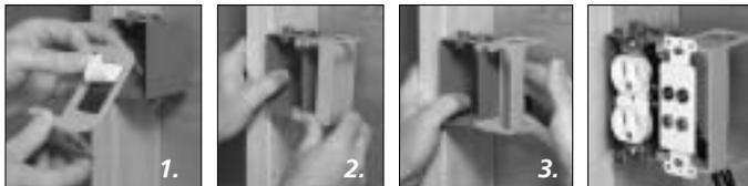
Attaching the Add-On Bracket is a "snap." You just remove the back of the double-sided tape (1), clip the bracket in place (2), and press on the bracket to secure it against the box (3). Allows for the installation of most decora style yoke plates
