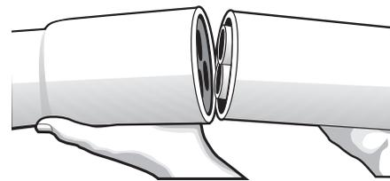
**3.** Raise both ends and align the innerducts on the male end into the coupling body on the female end. Lower both ends and the innerducts will automatically return to their original position as the joints are forced together.
