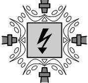
$\Delta \Delta$ Protected against water sprayed from a hose from all directions         |
