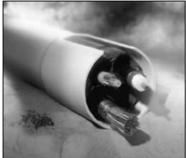
A 1/4" composite rope (braided polyethylene over braided polyester) was blown into the innerduct of Carlson's Multi-Gard. The force required to pull the rope through the 4,900 feet was 27 pounds. This force was measured after the rope rested in the flooded innerduct for more than 10 hours.
