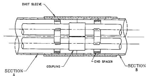
**2.** Align innerducts on Multi-Gard section "A" with couplings on section "B". Solvent cement each coupling for air tight seal and push until both ends are flush. Apply solvent cement to both ends of Multi-Gard and slide sleeve until it is centered on both sections.
