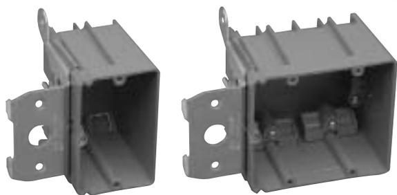
**The Carlon Adjust-A-Box** features a patented design that allows the box to be adjusted to most wall thicknesses with the turn of a screw. To install, simply clip the bracket onto the stud, secure with two screws to ensure the box won't move, then turn the adjustment screw clockwise or counterclockwise, and adjust the box flush with the wall covering.
