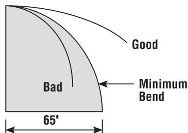
**Minimum Bend Radius:** Turns in a bore path should be made gradually. Bore-Gard and Boreable Multi-Gard have a minimum bend radius of 65'. Bending more than this recommended limit will stress the joint. The drawing below illustrates the 65' bend radius. To obtain a 90° turn you will require 65' of forward distance in any directional plane.
