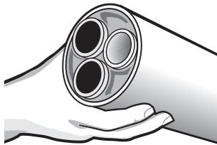
**2.** A spare spacer may be installed to align the innerducts if they seem loose.
