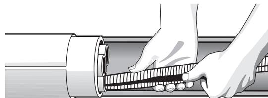
**2.** Install the 4" split sleeve couplings over the existing Multi-Gard. Slide the smaller split couplings onto the individual innerduct, fitting the cable into the split coupling. Repeat this process on opposite side. Carefully insert the cable(s) into the split corrugated innerduct.
