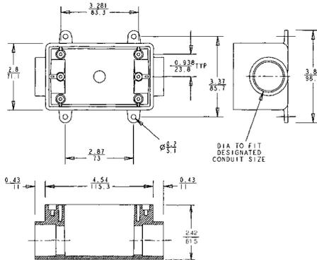
For through terminations where large devices or additional wiring capacity is required.
