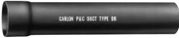
Carlton DB-100 nonmetallic P&C Duct Type DB is manufactured to NEMA Standard TC-6 & 8 and to specifications that exist within the State of California, and is designed for use in direct burial or concrete encased installations. Rated for use with 90°C cable.
