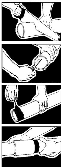
Carlton nonmetallic products are joined by means of solvent cement joints. Sizes 1/2" through 1 1/2" should be cut square (using a fine tooth handsaw) and deburred. For sizes 2" through 6" a miter box or similar saw guide should be utilized to keep the material steady. After cutting and deburring, wipe ends clean of dust, dirt and shavings.
