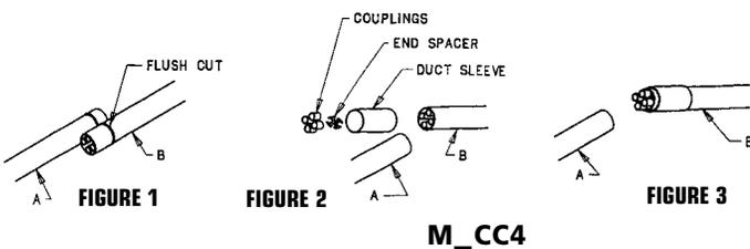
**1.** Flush cut Multi-Gard sections "A" + "B" as shown in figure 1. Slide outerduct sleeve over Multi-Gard section "B" as shown in figure #2. Insert end spacer into Multi-Gard plain end (chamfer side in) as shown in figure #2. Press couplings onto innerducts of Multi-Gard section "B" as shown in figure #3.
