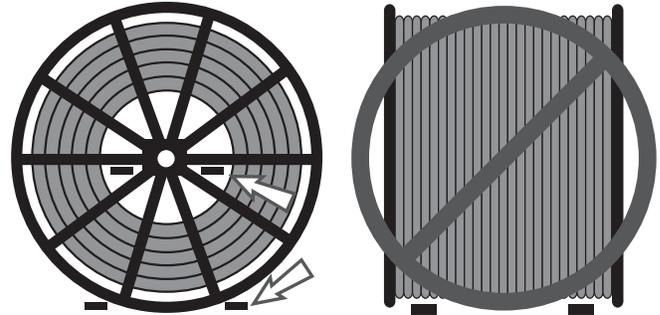
Reels must be lifted from the side with lift truck forks inserted through the spokes of the reel, or at the bottom with entry from the side of the reel. Reels should NEVER be lifted from the front of the reel or contact innerduct.
