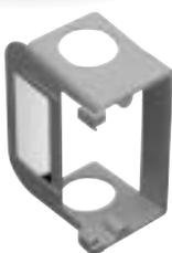
This low voltage bracket provides a low voltage outlet next to a previously installed high voltage outlet. Great for both new construction and rework, it attaches easily to most electrical boxes, and is designed to fit a standard two-gang faceplate. Resi-Rings accept 3/4" Resi-Gard only
