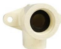
This elbow adapts from 1/2" CPVC to 1/2" male metal pipe threads and features lugs for fastening. A special elastomeric gasket ensures a leakproof seal. Used on tub and shower faucets to adapt from the 1/2" CPVC riser to the chrome shower arm. Sometimes called a "Drop Ear" elbow.
