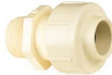
Designed to adapt from metal female pipe thread to PEX, copper, or CPVC tubing on the COLD WATER SIDE ONLY of a hot and cold water supply system.
