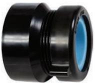
Utilized to adapt ABS pipe to tubular traps at wall or floor. This fitting solvent welds over 1½" DWV pipe. Sometimes called a Marvel.
