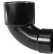
Used to change direction in piping as well as size. Usually utilized to convert from 3" horizontal pipe to 4" fitting hub directly under the toilet.
