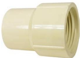
Used to adapt metal FIP threaded fittings to CPVC. A special elastomeric gasket ensures a leakproof seal. Hand-tighten only! This fitting seals by means of a gasket. The use of joint compound or Teflon tape is neither necessary or recommended.
