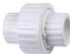
This union solvent welds directly to PVC pipe and provides a method for future disassembly of piping without cutting.
