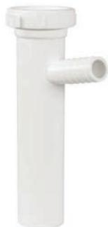
Used for hooking up automatic dishwasher drains to exposed sink drains in installations not employing garbage disposal. Branch accepts 7/8" I.D. hose or rubber dishwasher drain connectors
