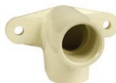
This elbow is used to change direction in piping and features lugs for fastening. Often used in conjunction with Washer Hose Valve (#530671) for hooking up to automatic clothes washers as well as fabricating water supply piping stub outs for toilet installation. Sometimes called a "Drop Ear" elbow.
