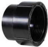
Conventional threaded cleanout fitting solvent welds into fitting hub and adapts to male threaded plug. PTFE thread tape is recommended for threaded joints.
