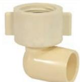
Allows a direct 90° connection between CPVC tubing and male running threads on faucet. Has a cone washer inside female end to achieve seal.
