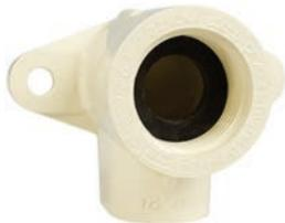
This elbow adapts from 1/2" CPVC to 1/2" male metal pipe threads and features lugs for fastening. A special elastomeric gasket ensures a leakproof seal. Used on tub and shower faucets to adapt from the 1/2" CPVC riser to the chrome shower arm. Sometimes called a "Drop Ear" elbow.
