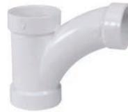
Required in some plumbing code areas to connect a branch line into a vertical drain pipe instead of conventional tee fitting. Also, used to connect a horizontal branch pipe approaching a horizontal drain pipe on the perpendicular.
