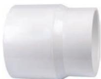
This fitting adapts Genova Sch. 40 pipe to 4" cast iron spigot and can be joined to cast iron with oakum and poured lead or poured lead substitute.
