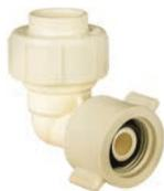
Allows a direct 90° connection between 5/8" O.D. PEX, copper, or CPVC tubing and male running threads on faucet. Has a cone washer inside female end to achieve seal.
