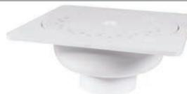
Designed to solvent weld to Sch. 40 IPS PVC. Installs easily and is direct replacement for cast iron and die cast bell traps. Outlet 3" Sch. 30 socket or 3" Sch. 40 spigot.
