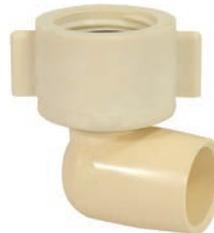
Allows a direct 90° connection between CPVC tubing and male running threads on faucet. Has a cone washer inside female end to achieve seal.
