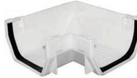
Used for either an inside or outside 90° corner. This support fitting is designed with seals and fitting marks that indicate the correct gutter placement to allow for expansion and contraction.
