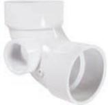
Used to connect a branch line or vent at a change of direction in a larger vertical or horizontal pipe. The inlet is constructed to accept a 2" fitting over its outside diameter or 1½" pipe into its inside diameter.
