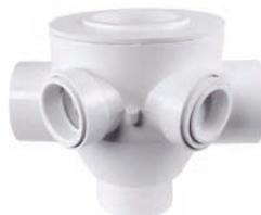
This special stack fitting provides for the hookup and venting of all drains from two complete bathrooms located back to back. Each unit includes two flush branch plugs to enable utilizing the fitting in a right or left hand drain situation. Branch inlets are 2" socket configurations to accept 2" pipe. Bushings (Part #70221) are provided to accommodate 1½" pipe.
