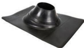
These weatherproof thermoplastic flashings, featuring a replacement boot, provide seal around plumbing vent pipes. Manufactured totally from corrosion proof materials. They eliminate shingle staining problems. Can be used on all types of plumbing pipes and electrical conduit. Base dimensions (14661) 8½" X 11¾", (14562-64) 12" X 16".
