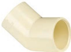
Used to change direction in piping. Sometimes used in conjunction with a 12" length of CPVC tubing on long runs to absorb expansion.
