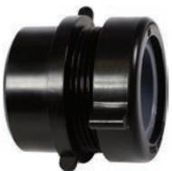
Utilized to adapt ABS fitting hub to tubular traps at wall or floor. This fitting solvent welds into a DWV fitting hub. Sometimes called a Marvel.
