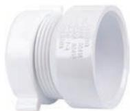
Utilized to adapt PVC pipe to tubular traps at wall or floor. Utilizes special washer which seals to either 1½" or 1¼" tubular products, reducing the number of SKU's needed in inventory. This fitting solvent welds over a 1½" DWV pipe. Sometimes called a Marvel.
