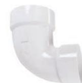
Used to change direction in piping as well as size. Usually utilized to convert from 3" horizontal pipe to 4" vertical pipe directly under the toilet.
