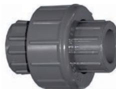
This union solvent welds directly to PVC pipe and provides a method for future disassembly of piping without cutting. Working Pressure: 150 PSI @ 73°
