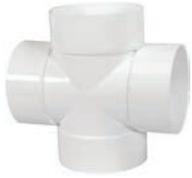
Used to connect two branch lines approaching a main sewer pipe from opposing directions. Used primarily in seepage bed grid in conjunction with perforated pipe.
