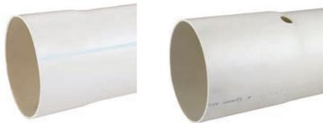
An integral hub is provided on each length of sewer and drain pipe to facilitate easy joining without the need for additional couplings. Pipe is perforated with 2 rows of 5/8" holes on 5" centers 120° apart. 3" Pipe is perforated with 2 rows of 1/2" holes on 5" centers 120° apart.
