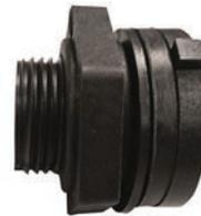
Polypropylene Bulkhead Fitting helps to permit the free flow of liquids for tank or drum drainage or filling. Includes EPDM washer. For use with tanks having a wall thickness of 1/16" to 1/2".
