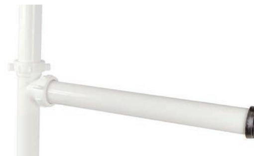
Fits any drain system. Designed to connect double compartment sinks that have a Garbage Disposal into a single trap. This unique unit can be assembled directly to sink strainer and disposal. Features a baffle in the tee to prevent back ups.
