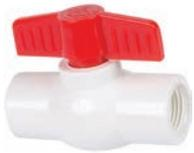
These ball valves are made out of PVC for corrosion resistance. Used anywhere a full flow valve is required, such as swimming pools, irrigation systems or agricultural applications. Adapts to standard male pipe threads. PTFE thread tape is recommended for threaded joints. Working Pressure: 150 PSI @ 73°
