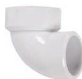
Used to change direction in "dry" portion of vent piping where water flow is not a consideration. Sometimes called a "Short Turn Street Quarter Bend".
