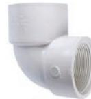
Used to change direction in piping. Adapts from solvent welded line to standard male pipe threads. PTFE thread tape is recommended for threaded joints.
