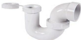
Used to prevent the passage of sewer gas from the plumbing system into house through the plumbing fixture drain. Used when local code doesn't permit the use of slip coupled traps.
