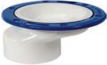
This flange has an adjustable metal ring which allows for easier toilet alignment. Used for mounting toilet base to drain pipe when pipe has been positioned incorrectly in installation.
