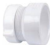
Adaptable 1½" x 1¼" washer included. Can be utilized to connect 1½" tubes, 1¼" tubes, as well as adapt from 1½" to 1¼" tubes. Solvent welds to 1½" Sch.40 drain pipe and connects via slip jamnut to either 1½" or 1¼" tubular traps. Eliminates the need for stocking extra trap adapter configurations.
