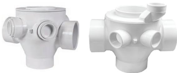
Provides for the hookup of all drains from two complete bathrooms located back to back. Each unit furnished with two flush branch plugs to enable utilizing the fitting in a left or right hand drain situation. Branch inlets are 2" socket configurations to accept 2" pipe. Bushing (Part #70221) are provided to accommodate 1½" pipe.
