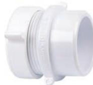
Adapts PVC fitting hub to tubular traps at wall or floor. Utilizes special washer which seals to either 1½" or 1¼" tubular products, reducing the number of SKU's needed in inventory. This fitting solvent welds into a 1½" DWV fitting hub. Sometimes called a Marvel.
