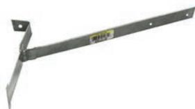
Used where fascia board does not exist or is not vertical. Attaches to roof under shingles. Connects to gutter brackets with Genova screws.
