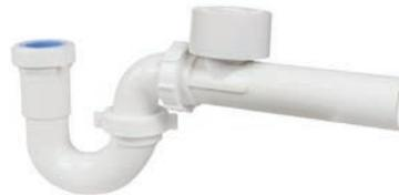
Combines the NovaVent™ anti-siphon valve and P-trap into a compact single unit. The anti-siphon trap provides a simple way of solving waste pipe drainage problems caused by inadequate plumbing system venting. Replaces almost any current fixture trap.
