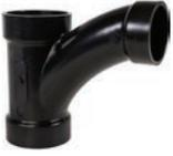
Used in some plumbing code areas to connect a reducing branch line into a vertical drain pipe instead of a conventional tee fitting. Also, is the acceptable method of connecting a horizontal branch pipe approaching a horizontal drain pipe on the perpendicular.
