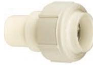
These patented adapters solvent weld directly into standard fittings and adapt mechanically to both PEX tubing and copper tubing by utilizing a special metal gripper ring supplied with the fitting. These fittings can be used in conjunction with CPVC fittings to create an unlimited range of fittings to connect to any type of water supply tubing.
