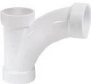
Required in some plumbing code areas to connect a branch line into a vertical drain pipe instead of conventional tee fitting. Also, used to connect a horizontal branch pipe approaching a horizontal drain pipe on the perpendicular. (Can be made from a wye and a "Street Eighth Bend").
