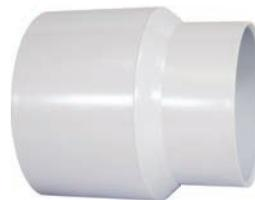
This fitting adapts 3" Sch. 30 pipe to 3" cast iron spigot. Can be joined to cast iron with oakum and poured lead or lead substitute.
