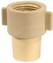
Allows a direct connection between supply tube and male running threads on faucet. Has a cone washer inside female end to achieve seal.
