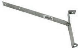
Used where fascia board does not exist or is not vertical. Attaches to roof under shingles. Connected to support brackets and slip joints with Raingo® screws.
