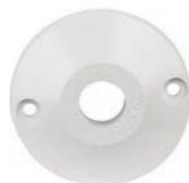
This special flange is designed to prevent torque change on CPVC pipes exiting through walls to which valves or threaded transition fittings are attached. The "torque flange" is welded to the pipe and fastened to the wall with screws thereby preventing twisting motion being transmitted to concealed joints.
