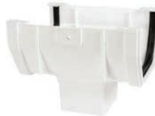
Used to connect Raingo® gutter with Raingo® downspout. This support fitting is designed with Raingo® seals and fitting marks that indicate the correct placing of gutter to give required expansion allowance.
