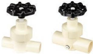
This unique valve employs the globe valve principle and is manufactured of high temperature thermoplastics. It is designed to solvent weld to CPVC tubing. This valve employs "Street/Socket" feature which allows it to be used with 1/2", 3/4", and 1" CPVC tubing. (2 - 3/4" couplings are required to attach the valve to 3/4" CPVC tubing. 2 - 1" couplings are required to attach the valve to 1" CPVC tubing).
