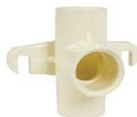
Used on lavatory and sink "rough-ins" instead of conventional tee, providing a more rigid "rough-in" and eliminates the need for tubing hangers. Also provides for rigid mounting of washer valves for automatic washer hose hook-ups at laundry tray.
