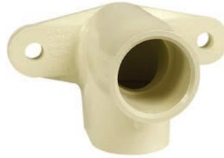
This elbow is used to change direction in piping and features lugs for fastening. Often used in conjunction with Washer Hose Valve for hooking up to automatic clothes washers as well as fabricating water supply piping stub outs for toilet installation. Sometimes called a "Drop Ear" elbow.
