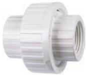
This union joins to male threaded pipe and provides a method for future disassembly of piping without cutting. PTFE thread tape is recommended for threaded joints.
