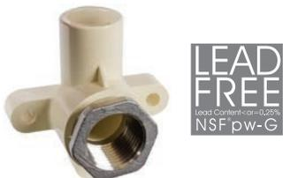
Used to transition from metal male pipe threads to CPVC. Provides for rigid installation by mounting elbow to wall. Usually used for shower arm or washer hose valve installation.
