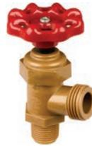
For use with female threaded fitting pipe in cold or hot water up to 150 PSI @ 180°F. (3/4" hose thread) PTFE thread tape is recommended for threaded joints.
