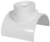
Solvent welds directly to side of sewer pipe to provide a simple way of connecting a branch into a drain pipe. The inlet is constructed to accept a 2" fitting over its outside diameter or a 1½" pipe into its inside diameter.
