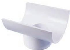
Solvent welds directly onto the side of a 3" pipe to provide a simple way of connecting a branch into a drain pipe. The inlet is constructed to accept a 2" fitting over its outside diameter or a 1½" pipe into its inside diameter.
