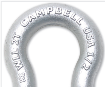
Date Code, "WLL" (Working Load Limit), "Campbell" or "CC", "USA" and size are permanently forged on shackle bow
