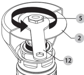
4. Place the new cutting disc **2** (not included) over the thread shaft.
