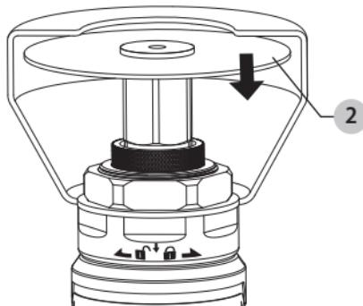
5. Place the washer on top of the cutting disc **2**. By hand, screw the hex nut **5** on by turning it clockwise. Use wrench **12** to tighten.
