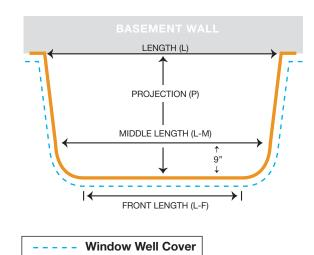
**NOTE:** Window well covers are made 2" larger than window wells to allow for some overlap.
