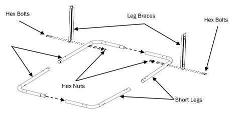
**Step 2:** Install Bottom Wire Shelf by placing the four corner hooks inside the hole on each leg then rotate the leg assemblies up and secure the Leg Braces to the other side of the Long Leg and Short Leg set.
