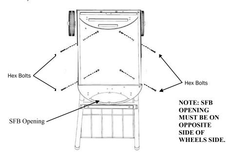
**Step 5:** Install SFB to the Grill Body using six 1/2" Hex Bolts, two 2" Hex Bolts, and eight Hex Nuts. Bolts should go through the holes from the inside of the SFB Body.
