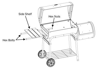
**Step 8:** Attach Front Shelf to Grill Body with four Hex Bolts and four Hex Nuts. First Assembly the side shelf using four 1" Carriage Bolts and four Hex Nuts.
