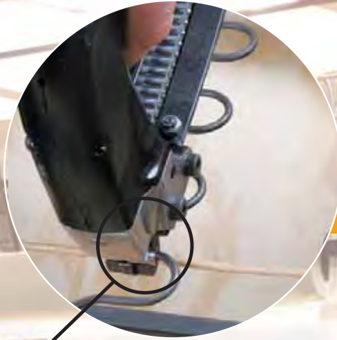
HR-66C-110 Clip Tool connecting tie wire to sinuous springs
