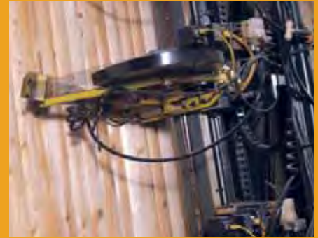
Machine mounted nailer applying Fencer Plus™ Nails
