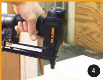
Caseback being secured with 18-gauge SL staples
