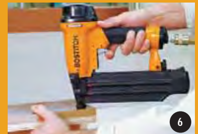
16-gauge nails securing a cabinet face
