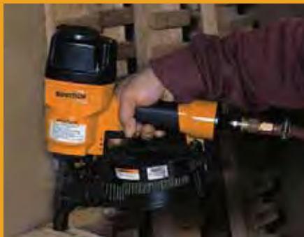
N58C Coil nailer fastening fence header board
