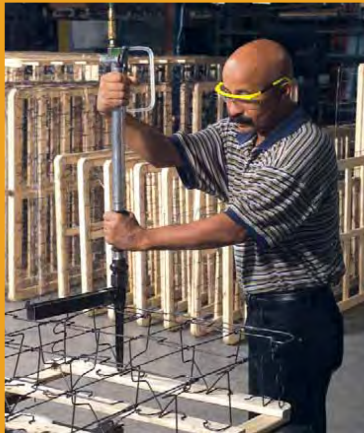
BCAR-2S Stapling foundation spring to flat
