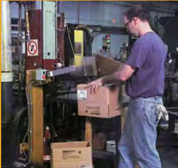
FC95EC Bottom closer used to clinch carton bottoms
