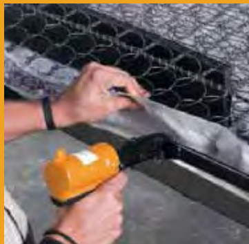
TR203 D-Ring tool connecting flange to innerspring
