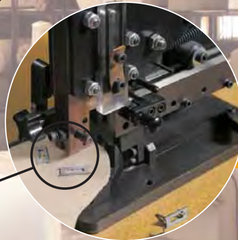
LockNail™ Machine applying LockNail™ to upholstered panel
