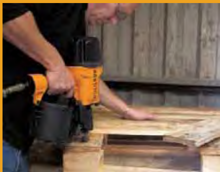
N400C-1 Nailing mat to block pallet
