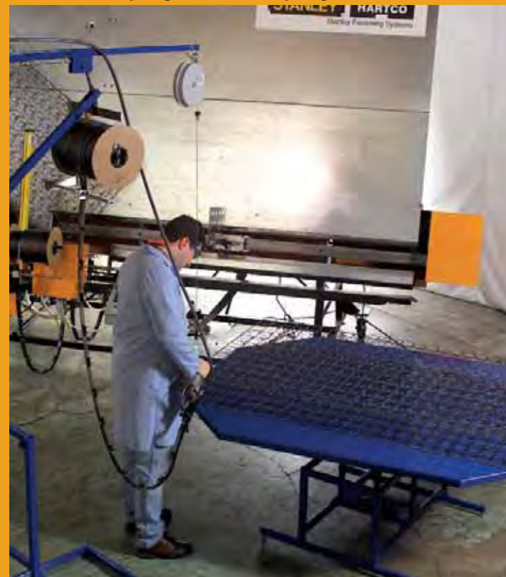
Coil clip system and vertical rotating clip machine securing innersprings to borderwire
