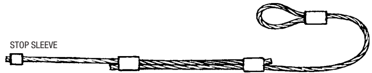
LAP SPLICE - OVAL SLEEVES OR DUPLEX
