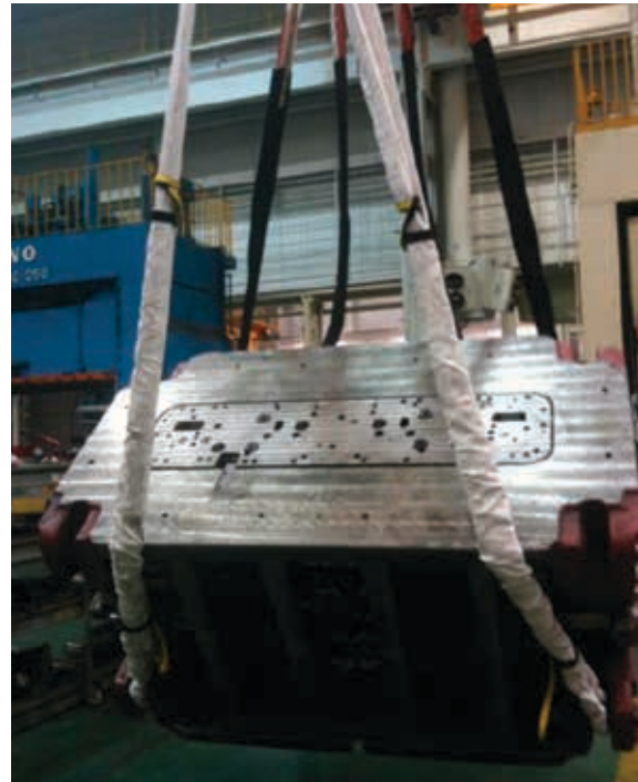
Wear pads made with Dyneema® yarns flipping a mold
