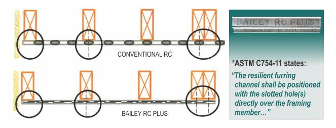
Incorrect positioning with other designs of resilient channel has resulted in a reduction in performance of 1-3 STC points. Common conditions where the required positioning is a problem with conventional designs, is not an issue with the Bailey **RC PLUS**.
