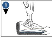
Attach mop pad by wrapping around bottom of foot, making sure gray stitching is located on the front of foot and the Quick Grip Release Tab is located on the back.
