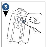
To fill the water tank, remove grey rubber nozzle on the back of the water tank.
