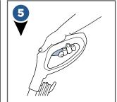
Push the trigger on the handle to release steam.
