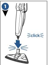
Attach lower body to mop pad foot by snapping it into place.
