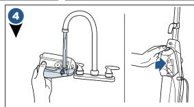
Fill water tank with distilled or demineralized water, recommended in place of tap water. Place the nozzle back into the water tank after filling and return tank to machine.
