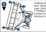
Unplug and turn vacuum over. Unscrew 7 Phillips head remove cover.
