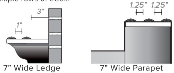
Bird Jolt Flat Track® easily glues in place with construction grade adhesives. Installation requires general knowledge of electrical systems. If you have questions or need an Authorized Installer call us at 800.392.6915.
