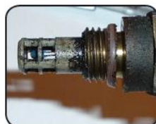
Temperature Sensors Covered with Soot
