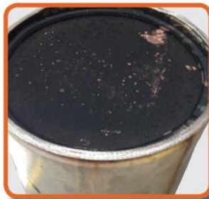
Diesel Particulate Filter Clogged with Soot
