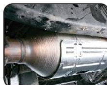
Diesel Particulate Filter Clogged with Soot
