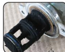
Dirty EGR Valve Clogged with Soot
