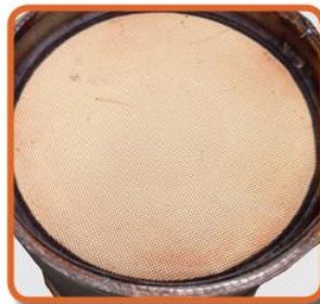
Diesel Particulate Filter Clogged with Soot
