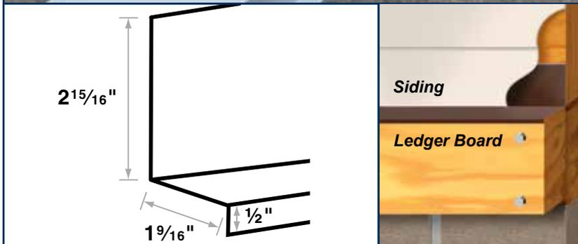
Technical drawing dimensions:  $2\frac{15}{16}$ " height,  $1\frac{9}{16}$ " base width,  $\frac{1}{2}$ " lip thickness.
