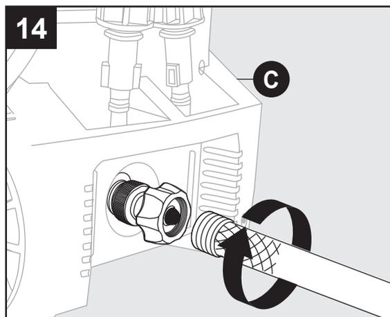
Attach a standard garden hose to the black collar of the garden hose adapter located on the back of the power washer unit (C). The water is now connected to your power washer.
