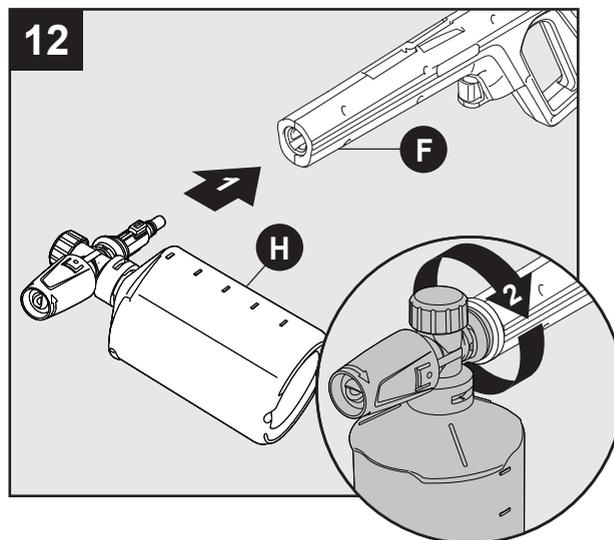
Insert foam cannon (H) into spray gun (F), push in and turn clockwise.
