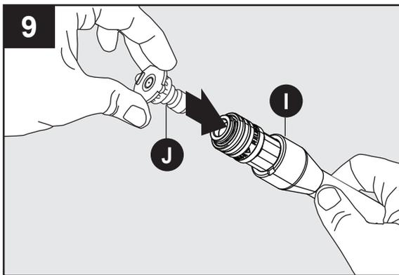
Attach nozzle (J) into end of lance (I) by pressing selected nozzle into place. It will make a “click” sound when firmly in place.
