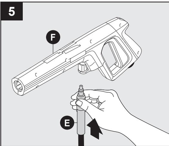
Connect the other end of Super Soft high pressure hose (E) to spray gun (F) by inserting the silver metal tip of Super Soft high pressure hose into the fitting just ahead of trigger guard. It will lock into spray gun with a “click”. Confirm hose is locked into spray gun by slightly pulling on hose. The hose is now securely attached to spray gun.
