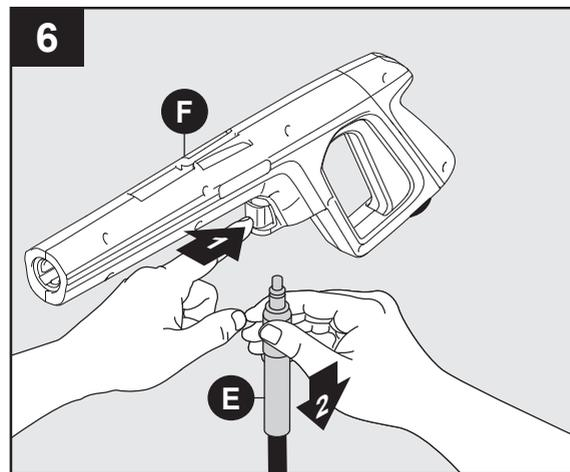
To release hose (E) from spray gun (F), press button on underside of gun toward trigger guard. The hose will slide out from connection.
