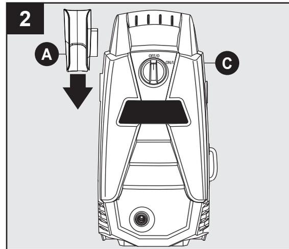
Slide spray gun holster (A) onto left side, when facing the power washer unit (C) as shown.
