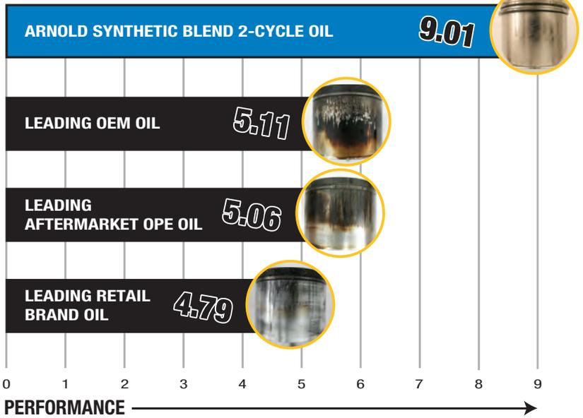
50 Hour Detergency Wear Test. Used Troy-Bilt TB32 Weed Trimmer 25cc engine, each test conducted with new unit.
