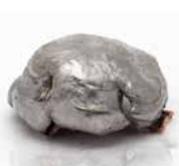
9mm 124gr. 98% weight retention 1200 fps
