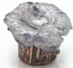
9mm 124gr. 98% weight retention 900 fps
